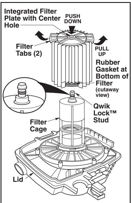
**NOTE:** This filter is made of high quality paper designed to stop very small particles of dust. The filter can be used for wet or dry pick up. Handle the filter carefully when removing to clean or installing it. Creases in the filter pleats may occur from installation but creases will not affect the performance of the filter.
