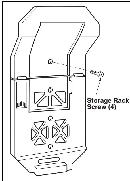
**▲ CAUTION:** To prevent plywood, Storage Rack, or Wet/Dry Vac from falling, make sure you have selected the proper length of fastener for the secure mounting of storage rack to the wall.
