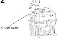
Press the switch button to turn on/off the cleaner
