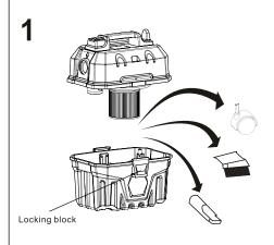
Release the lock block to open the Upper housing, then take out wheels and other accessories.
