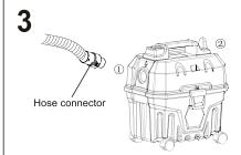
Put the hose connector into ①,the suction fucntion is available Put the hose connector into ②,the blow fucntion is available
