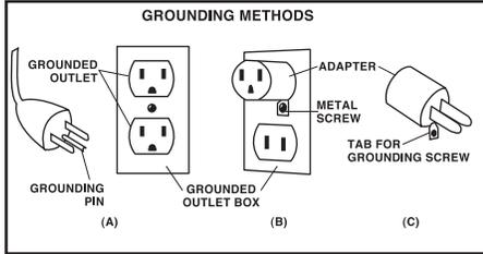
IN CANADA, THE USE OF A TEMPORARY ADAPTOR IS NOT PERMITTED BY THE CANADIAN ELECTRICAL CODE. Make sure that the appliance is connected to an outlet having the same configuration as the plug. No adapter should be used with this appliance.
