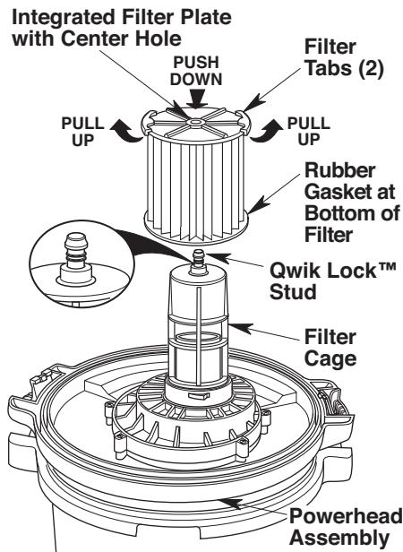
**NOTE:** Failure to properly seat the bottom Gasket could result in debris bypassing the Filter.
